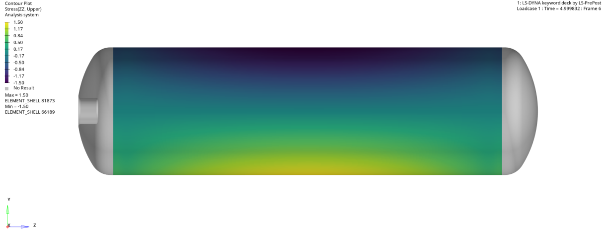
Figure 6.14: Normal stress \sigma_{zz} due to effect of gravity: Numerical Model.
