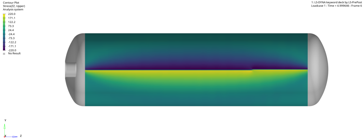
Figure 6.7: Numerical longitudinal stress \sigma_{zz} under step-wise thermal gradient (tank with normally stiff heads).
