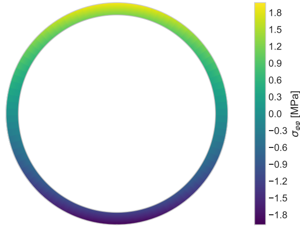
Figure 6.12: Analytical circumferential stress \sigma_{\varphi\varphi} for temperature profile B.
